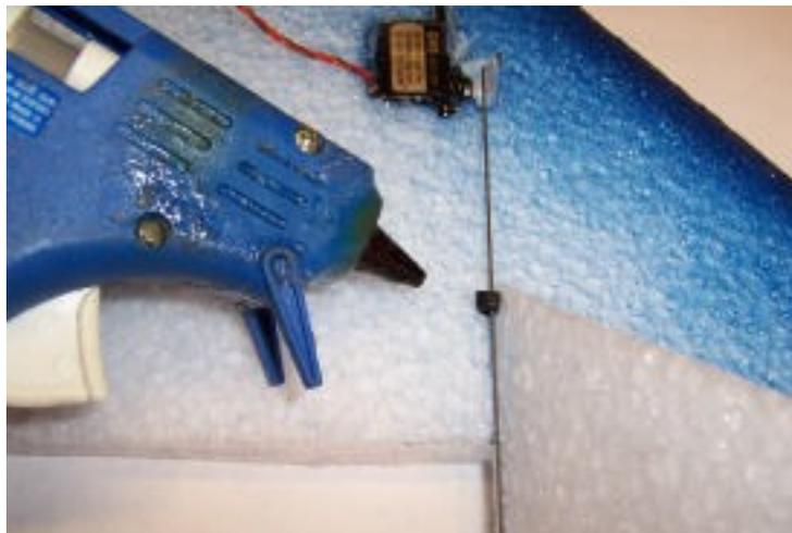
Make a "L" bend on pushrod at control horn and secure with EZ Link.
