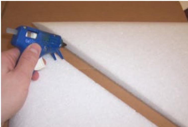
With the wings glued together, it is time to install the elevons. Place the elevons on the correct side of the wing and leave approximately  $\frac{1}{4}$ " -  $\frac{1}{2}$ " of space between the elevons at the center of the wing. With the gap between the elevons, you will have some overhang on the tips of the elevons - we will cut this off after the elevons are glued on. The elevons come beveled, make sure the beveled side goes "down."
