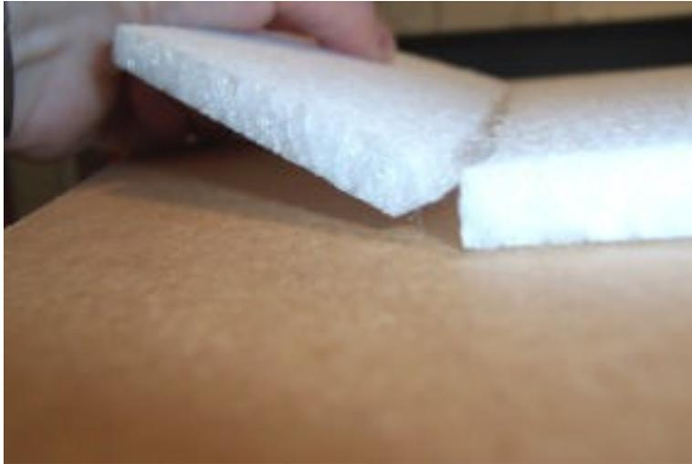
Now comes the time to glue the elevons down. Perhaps the best glue for an EPP to EPP hinge is Welder glue. If you do not wish to use Welder, hot glue works very well, also. Once you choose the glue you'd like to use, the elevons must be lined up onto the wing. The 45 degree bevel needs to be facing down along trailing edge of plane. Also ensure there is no gap at the hinge line and choose one of the following methods:
