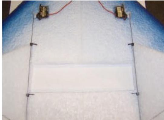
Install "Z" bends into servo arms. Center servo arms and position servos so that the pushrod almost touches the inside of the fins. Elevons should be flat on the bench. Push zip ties into foam and secure with a small amount of hot glue.
