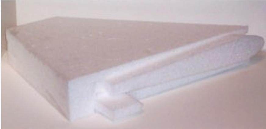
Save the sheet of foam from between the wing halves. Gently rub wing halves together to remove any slag. Do the same with elevons. Glue the wing halves together with hot glue or Welder glue on a flat surface. Make sure to orient the wing properly. The flat side of the wing is the bottom.
