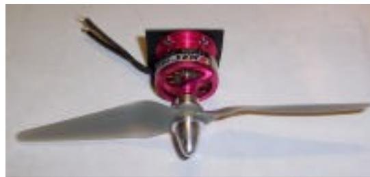
Use hot glue to secure motor mount assembly onto the canopy as shown. Motor should be centered on the canopy as viewed from the top. Position motor up slightly away from where it may touch the airplane.
